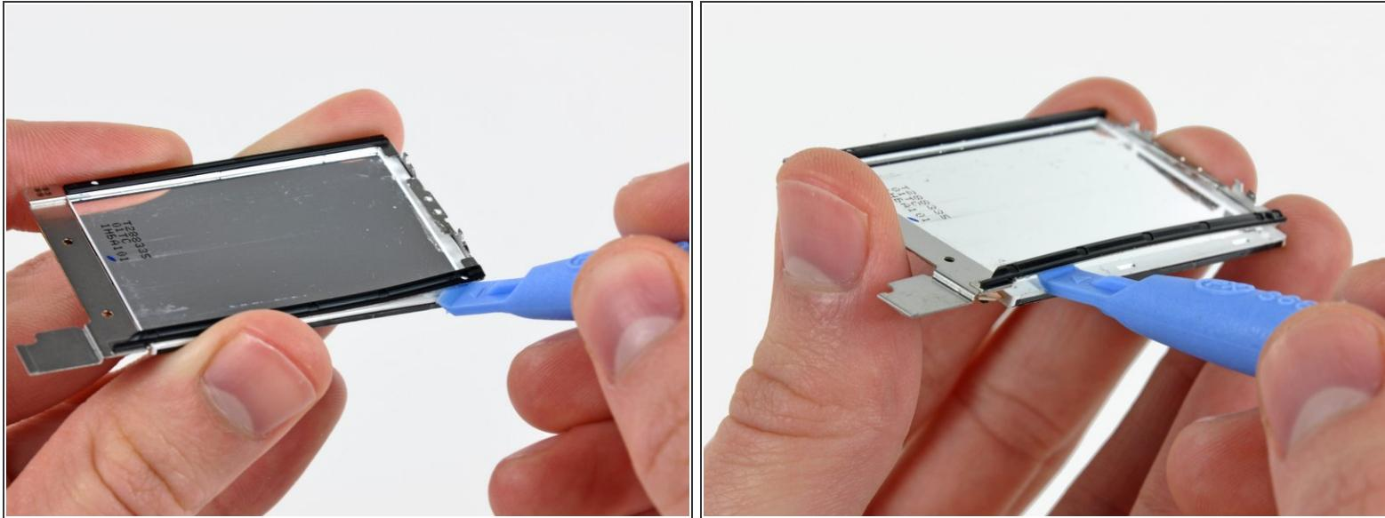
*(i)* The display bracket is attached to the display by a strip of adhesive around its perimeter.
